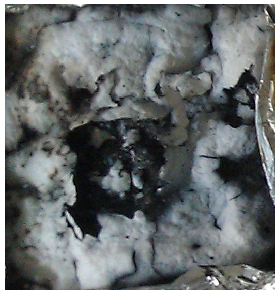
Figure 6. Image of residue of CONE test. [Color figure can be viewed in the online issue, which is available at wileyonlinelibrary.com .]
