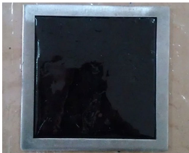
Figure 3. Preparation of test slice for CONE test. [Color figure can be viewed in the online issue, which is available at wileyonlinelibrary.com .]
